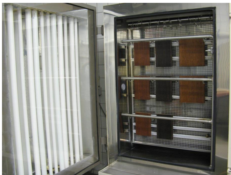
Fig. 1: Positioning of test specimens in the weathering chamber
